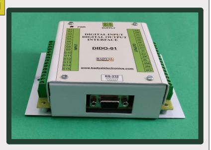
Digital Input & Output Module offers robust and versatile digital signal processing capabilities for industrial applications. With support for a wide voltage power supply range of DC 7 to 36V, it ensures compatibility with various power sources commonly found in industrial environments. It offers 15 Input CH for interfacing with external sensors. 15 output CH utilizes Darlington transistors, provides stronger driving capability with up to 500mA sinking current, built-in flyback diode protection
